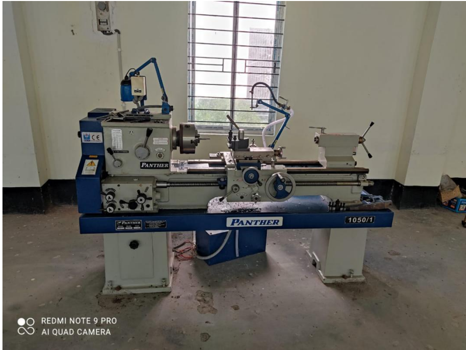
Figure 2: All geared precision lathe machine.
