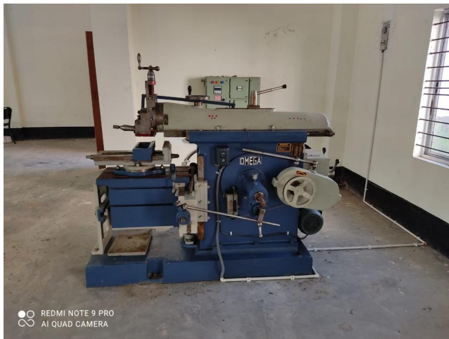
Fig 1: Heavy Duty all geared Shaping machine
